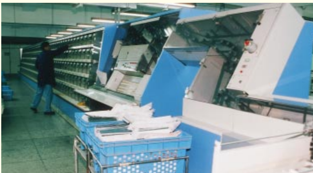
光學閱讀分揀機 Optical character reader / letter sorting machine
